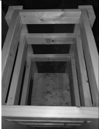
I used 2 x 4s to give structure to the frame.
